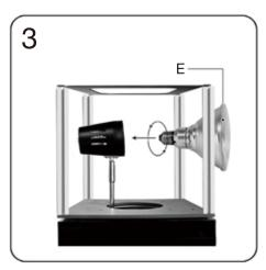
Screw in a halogen bulb in the bulb socket.
