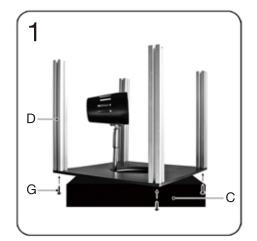
Fix aluminum frames on the base with screws.
