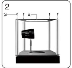
Fix the top plate at the top of the aluminum frames with screws.
