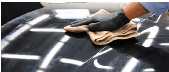
Unevenness of coating caused by waiting too long
