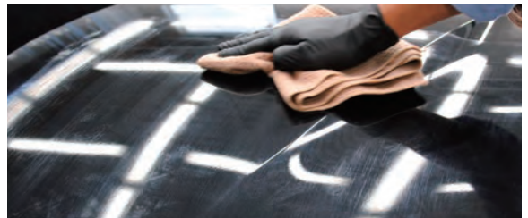
Unevenness of coating caused by waiting too long
